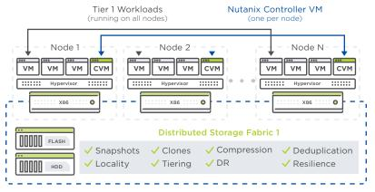
Figure 3. Acropolis Distributed Storage Fabric joins HDD and SSD resources from across a cluster into a storage pool
