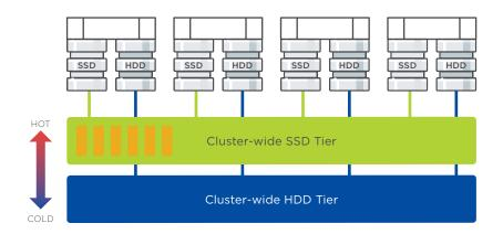
Figure 4. VM Flash Mode allows individual  $\nu$ Disks to be "pinned" in the cluster-wide SSD tier for maximum IOPS and low latency.
