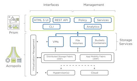
Figure 14. High-Level Prism Architecture.
